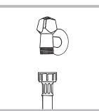
2. Connect the inlet hose by screwing it to a cold water tap using a 3/4 gas threaded connection (see figure).
